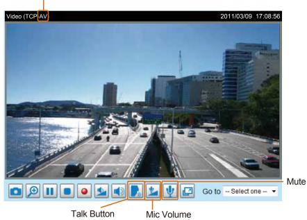
Audio is being transmitted to the Network Camera
